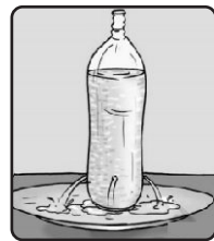
Liquid exerts the same pressure in all directions at given depth.
